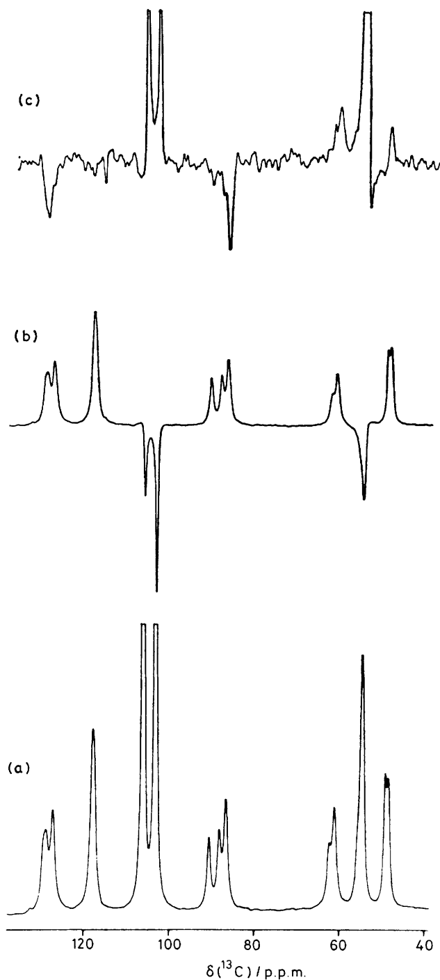
Figure 1. (a) A partial 100.6 MHz 13 C n.m.r. spectrum of \text{Fe}(\eta^4\text{-C}_8\text{H}_8)(\text{CO})_2(\text{CNPr}^i) in \text{CD}_2\text{Cl}_2\text{-CHFC}_l_2 , 1:1, at -118^\circ\text{C} . In addition to the cyclo-octatetraene signals, there is a doublet at \delta 104.9 due to \text{CHFC}_l_2 , a weak doublet at \delta 89.5 due to solvent impurity coincident with the signals due to carbons a' and a'' , a broad singlet at \delta 54.6 due to \text{CD}_2\text{Cl}_2 , and two signals at \delta 49.2 and 48.4 p.p.m. due to the methine carbons of the isopropyl group. (b) The partial spectrum 1 \mu\text{s} after applying a selective 180^\circ pulse at \delta 55.5 p.p.m. A sideband, 5 kHz away perturbed the \text{CHFC}_l_2 signal. (c) A difference spectrum obtained by subtracting spectrum (b) from that obtained 10 ms after applying a selective 180^\circ pulse at \delta 55.5 p.p.m.
